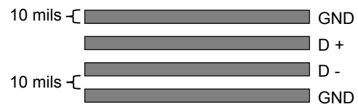
Figure 13 Recommended Remote Diode Circuit Board Interconnect
